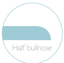
Step tread 20mm Typically 600 x 100mm
